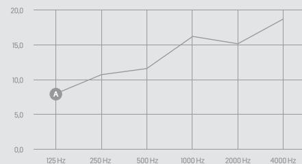
Cone screens have the best properties of sound attenuation. The average attenuation according to ISO 10053 is 15dB.
