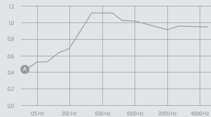
[x] Frequency [Hz] : [y] Sound absorption coefficient [as]
