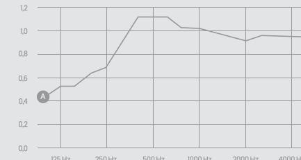
[x] Frequency [Hz] : [y] Sound absorption coefficient [αs]
