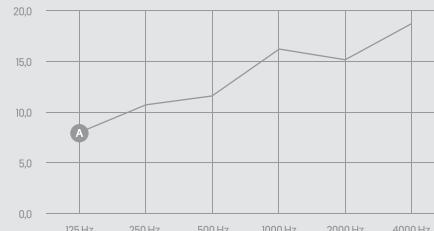
[x] Frequency [Hz] : [y] Sound attenuation [dB]
